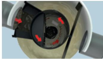
Stormwater carrying litter, suspended solids, organic matter and oils flows into the central Treatment area where a vortex effect is used to capture those pollutants. The floatables are kept in this central treatment area.
