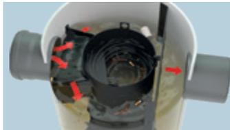
During high flows when the overflow is active, the outlet baffle plate ensures new floatables are still captured.
