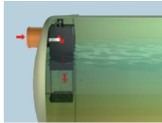
Polluted stormwater flows into the Stormsed. The inlet design distributes flow evenly across the device and protects already captured sediment.
