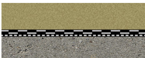
Balcony with waterproofing membrane, reversed roof
